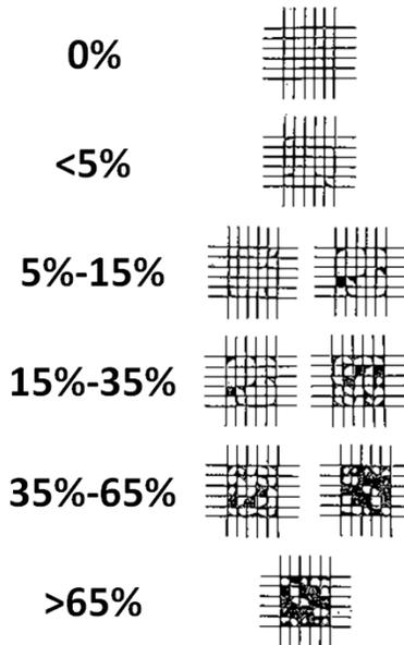
**FIGURE 2: MATERIAL LOSS FROM ADHESION TESTING (ADAPTED FROM ASTM 3359)**
